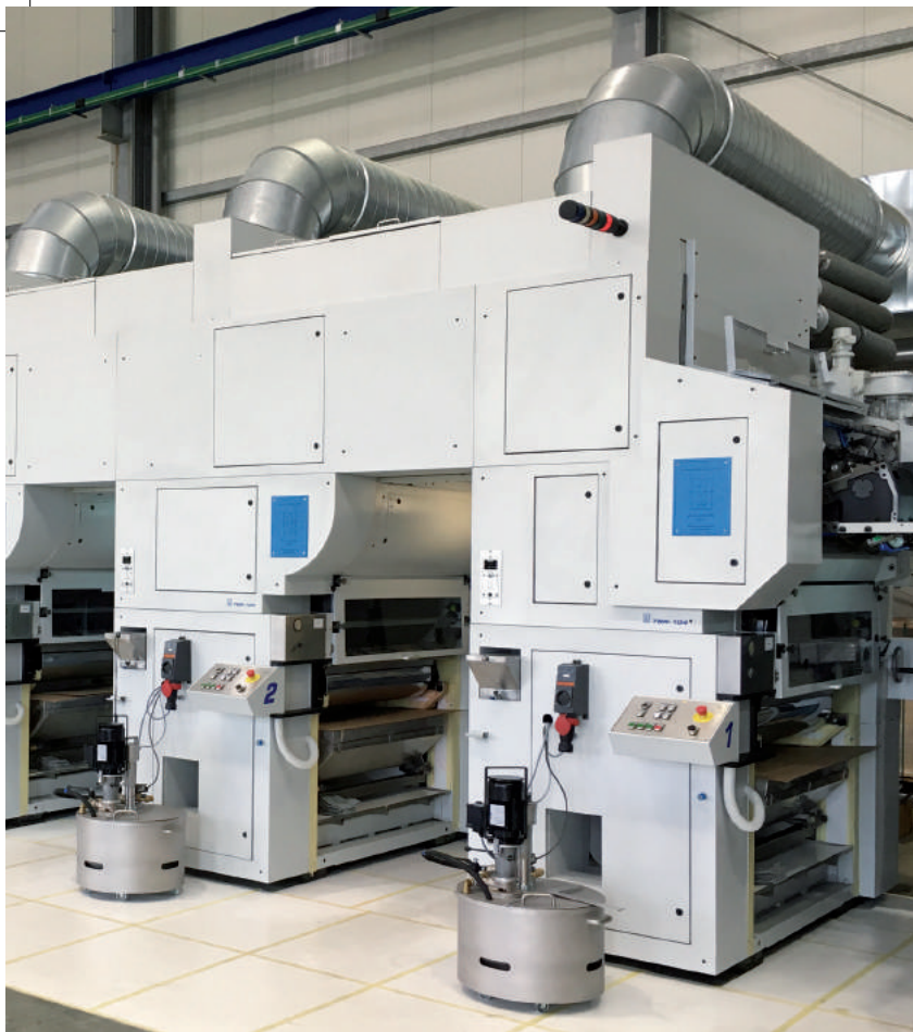
The TBR-104 is a sheet-fed gravure printing press for the printing and finishing of packaging with high quality standards
